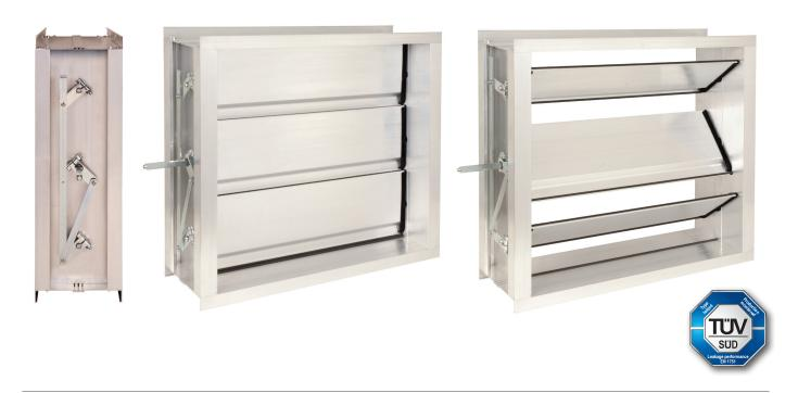
The APS Arosio damper without plastic parts is a special version suitable for special environment (like low/high temperature, chemical agents) where it is not possible using the polypropylene gear mechanism. The blades and the frame are in extruded aluminium and it can be supplied with actuator (mounting bracket for motorised movement).
